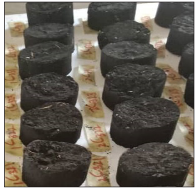
Figure 3. Produced briquettes from sawdust and cassava peel materials
